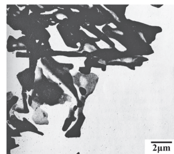
Fig. 10 TEM image of cross section in region D ( V=240\mu\text{m/s} , G=11^\circ\text{C/mm} ) 4) .
