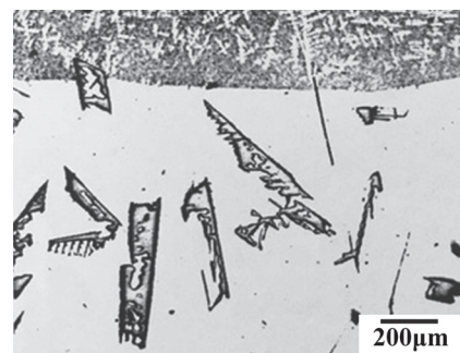
Fig. 3 Observation of solid-liquid interface (longitudinal section) in region A ( V=0.28\mu\text{m}/\text{s} , G=30^{\circ}\text{C}/\text{mm} ) 3) . 領域 A ( V=0.28\mu\text{m}/\text{s} , G=30^{\circ}\text{C}/\text{mm} ) における固液界面の観察 (縦断面) 3) .
